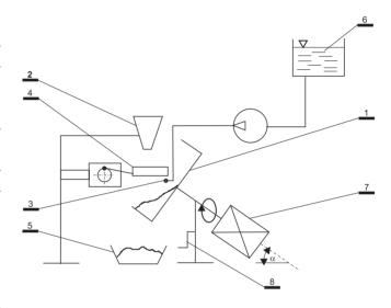
FIGURE 1. Scheme of the stand for pressureless granulation (1 - granulator's tray, 2 - supply of the material, 3 - spraying nozzle, 4 - sieve, 5 - final granulate, 6 - binding liquid, 7 - motor, 8 - crank for adjusting the tray inclination).
