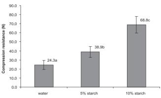
FIGURE 5. Compression resistance of granulated dried mushrooms depending on binding liquid.
