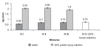
FIGURE 4. Mean size of granulate for particular mixtures.
